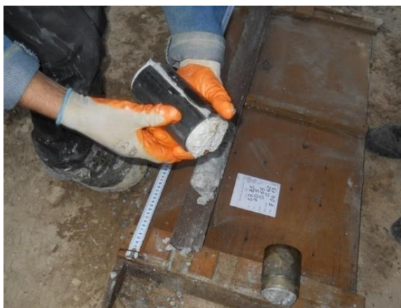
Packing a sample by a plastic half-tube.
